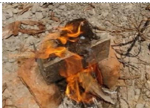
Figure 6. Papercrete brick during fire test.
