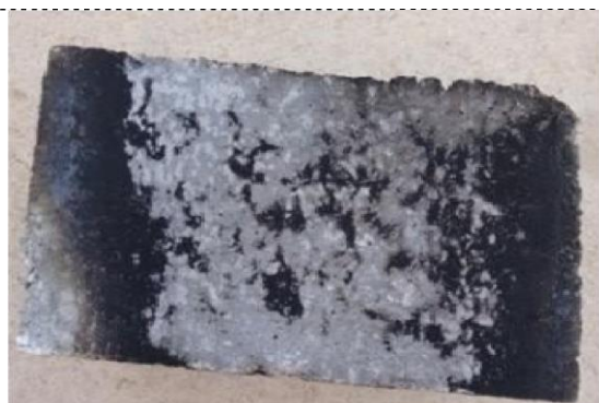
Figure 7. Papercrete brick after fire test.
